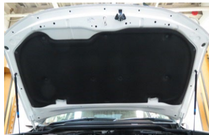
Automotive sound-absorbing material "Hood insulator"
