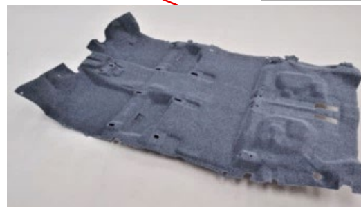
Automotive sound-absorbing and sound-insulating materials "Floor carpet"
