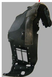
Automotive sound-absorbing material "Front wheelhouse liner"
