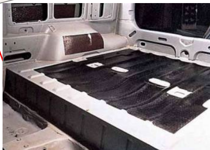
Automotive vibration-damping material "MELSHEET"
